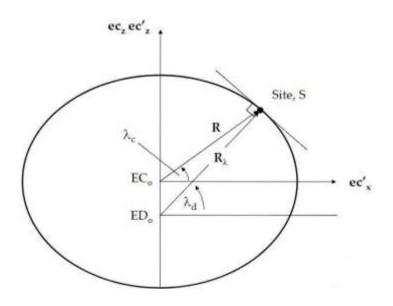
Figure 2.2 Cross-section of the earth [17].
