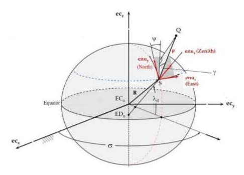
Figure 2.1 Topocentric Coordinate System ([14] as adapted by [17]).
