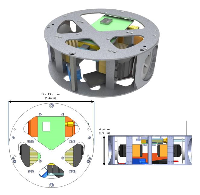
Figure 15. New, miniaturized System V.2 steering control architecture.
