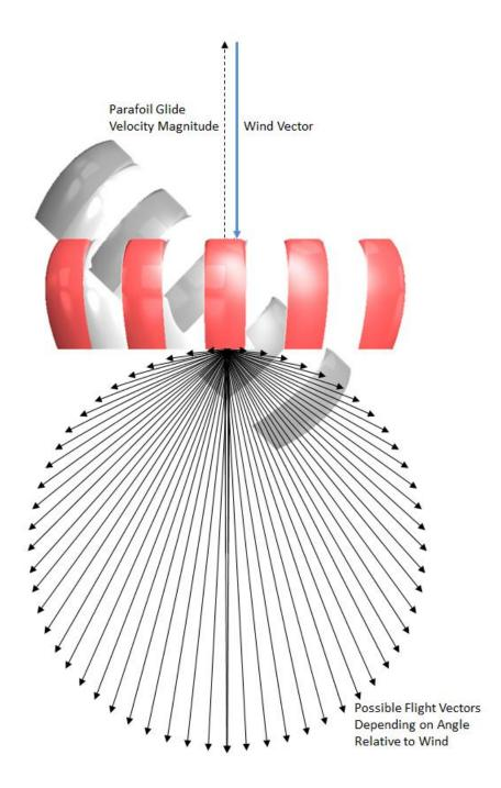
Figure 33. Range of possible flight vectors, when wind velocity is exactly equal to parafoil glide velocity. No forward progress is possible, and lateral flight vectors are extremely limited in magnitude. As wind speed dominates, the ellipse of possible headings narrows further in width and stretches in height (vertically).
