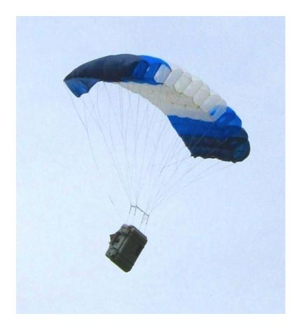
Figure 3. The advanced, high-precision, miniature Snowflake Aerial Drop System.<sup>8</sup>
