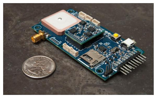
Figure 21. Ryan Mechatronics Monkey Cortex Navigation Platform. The miniature board has a programmable microprocessor, microSD card data logging, GPS, 6 PWM servo outputs, and a socket to accept a plug-in 3-axis IMU roughly the size of a postage stamp.
