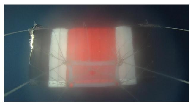
View from the up-looking camera after successful parafoil inflation at 50,000 ft. altitude ASL. The parafoil has already stabilized into a very steady flight path with the wind vector.
