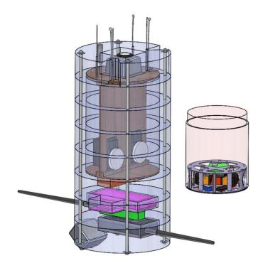
Figure 17. Old System V.1 architecture (left) compared to new System V.2 architecture (right). The transparent red cylinder around System V.2 indicates the remaining available payload volume for parafoil stowage and deployment systems.
