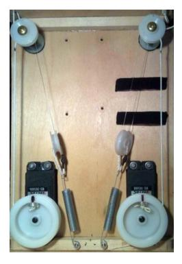
Figure 14. Volumetrically-inefficient System V.1 line tensioner configuration.
