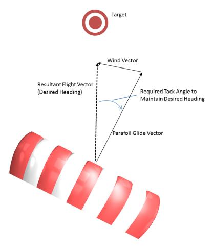
Figure 32. Relationship between wind vector, desired heading vector, and parafoil system orientation to maintain flight path toward target.
