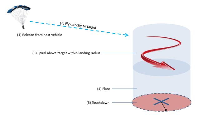
Figure 25. Pictorial concept of operations for flight software control scheme.
