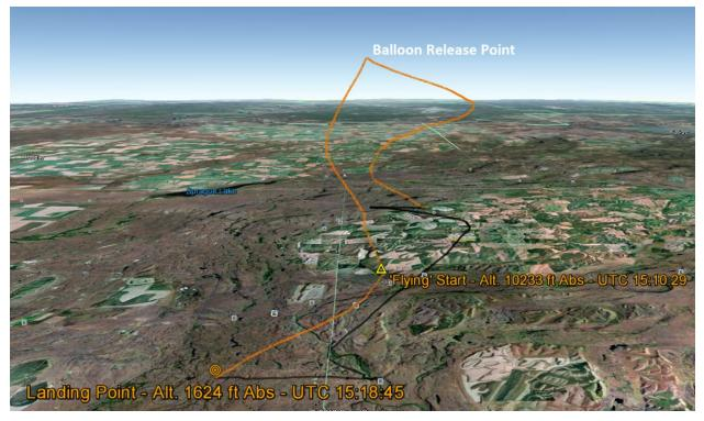
Figure 8. GPS-logged flight track of parafoil system during Balloon Flight Test #2. The nominal due-west flight for the last 10,000 ft. of descent can be seen in the ground-track shadow.
