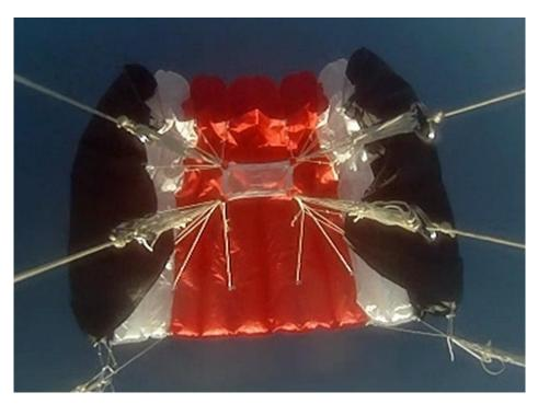
Figure 7. Partially-inflated parafoil and elevated bridle resulting in loss of control during first 23,000 ft. of descent during Balloon Flight Test #2.
