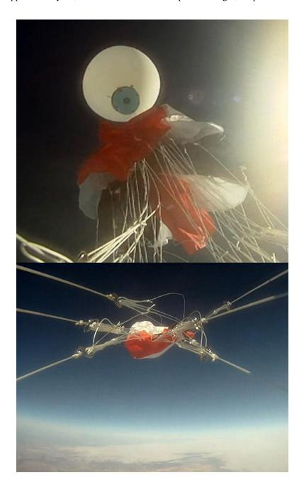
Figure 9. Top: Immediate collapse of parafoil following balloon separation in Flight Test #3. Bottom: Flat spin resulting from collapsed parafoil proves to be unrecoverable.
