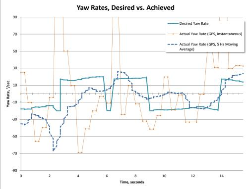
Figure 44. (5 plots, above) Typical flight performance data for the first iteration of the steering software. At no point was it able to consistently steer toward the target coordinates.
