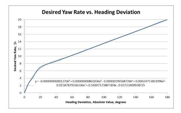
Figure 34. Yaw rate curve for control algorithm. As deviation from desired heading approaches 0, the system strives to achieve a yaw rate of  $0^{\circ}$ /s. At greater deviations, the desired corrective yaw rate scales proportionally. A  $6^{\text{th}}$  order polynomial curve fit is used as the input to the steering software algorithms.
