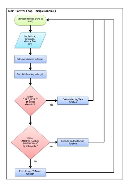
Figure 26. Flow chart of the main control loop of the System V.2 control software.
