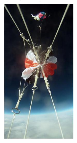
Figure 6. The tangled parafoil co-orbits the steering system in a flat spin during Flight Test #1.
