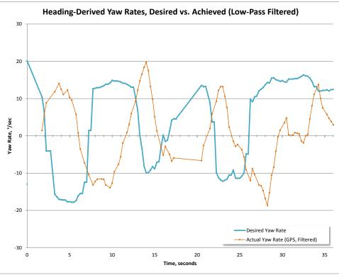
Figure 48. (5 plots, above) Flight performance data for the third iteration of the steering software, in moderate wind conditions. These results are improved over the prior set of plots due to an increased steering gain value being used. However, the parafoil control response is still slightly delayed, as seen in the yaw rate plots.
