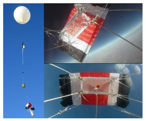
Figure 11. Left: Rigidized parafoil maintains its shape beneath balloon payload train. Top Right: Rigidized parafoil structure *immediately* inflates upon separation from balloon at 42,000 ft. altitude, but a line snag causes an uncontrollable spiral. Bottom Right: Rigidized parafoil in nominal flight after snag is freed at approx. 3000 ft. altitude.
