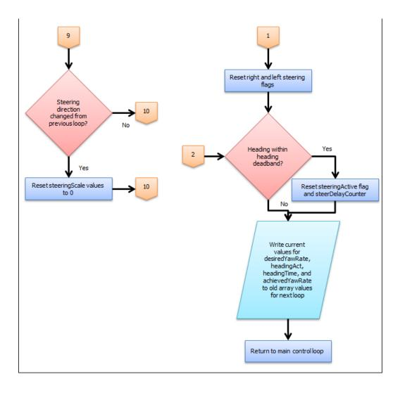
Figure 27. (Previous page and this page.) Flow chart of the steerToTarget control routine of the System V.2 control software.
