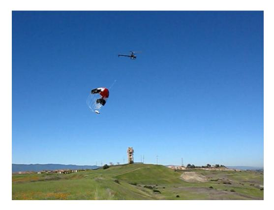
Figure 38. Video capture of parafoil being lifted by the R/C helicopter for one of many drop tests.
