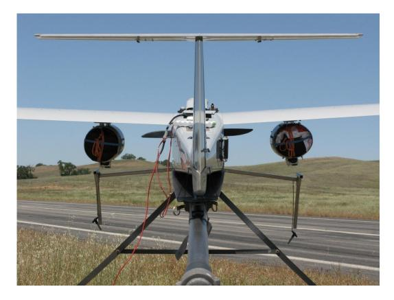
Figure 41. System V.1 (left) and System V.2 (right) mounted to the wings of the UAV, ready for flight.
