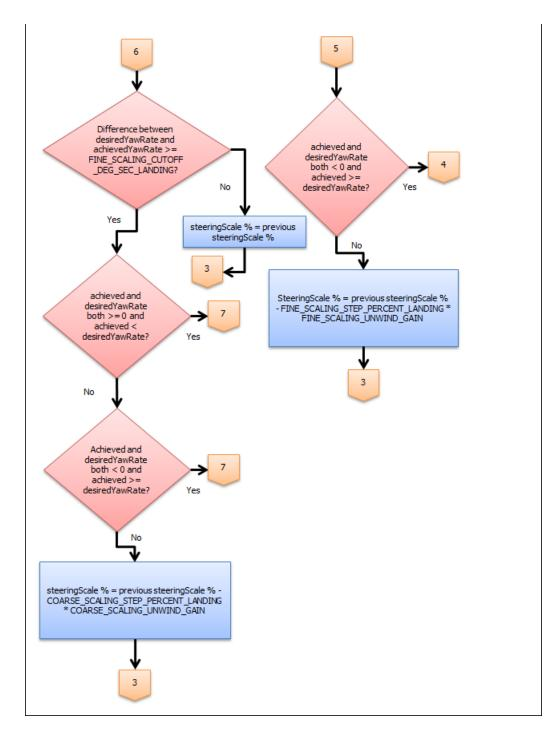
Figure 30. (Previous page and this page.) Flow chart of the steer scaling sub-routine of the landing routine for the System V.2 software.
