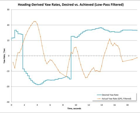
Figure 46. (5 plots, above) Flight performance data for the second iteration of the steering software, in moderate wind conditions. Note the two major spikes in the heading deviation plots. These are the result of light wind gusts, and the parafoil system's response is much too slow to compensate.
