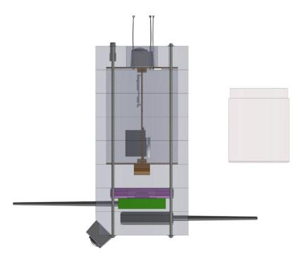
Figure 12. Existing System V.1 balloon test system (left) compared to available volume for both the SPQR-specific System V.2 *and* its parafoil stowage.
