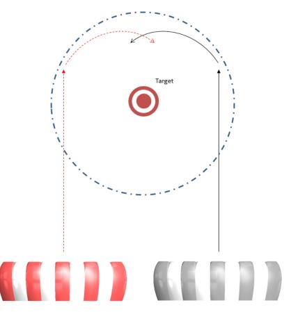
Figure 35. Determination by the landing routine of the sense of the appropriate yaw rate vector.
