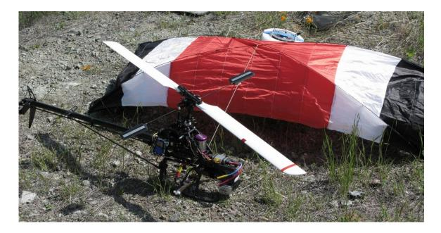
Figure 37. R/C helicopter used for lifting, and System V.2 prior to drop testing.
