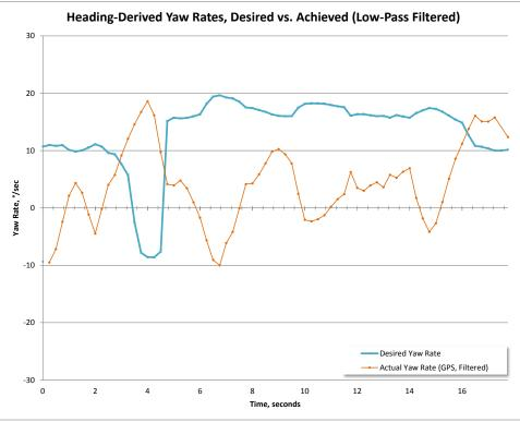
Figure 47. (5 plots, above) Flight performance data for the third iteration of the steering software, in moderate wind conditions. These unimpressive results are due to the steering gain (the rate of servo stepping per loop) being set too low. For this flight, a servo step of 12% of maximum pull, per second, was used.
