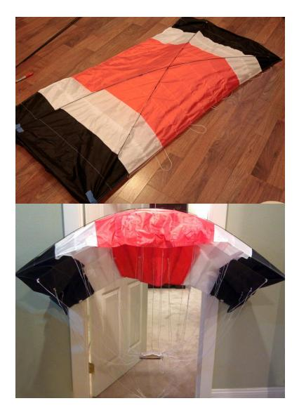
Figure 10. Top: Parafoil stiffening structure test-fitted to parafoil. Bottom: Suspended parafoil remains open, yet highly flexible under its own support.
