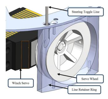
Figure 18. Detail of the structural ring (shown transparent) used to keep the steering toggle line captive in the servo wheel. This ring eliminates the need for a volumetrically inefficient, mechanically complex tensioning system.
