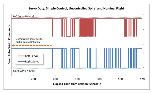
Figure 23. Servo actuation pulses during a descent from 27,000 ft., used to approximate servo duty cycles as a percentage of total flight time. The first 390 seconds of this flight were an uncontrolled spiral due to partial parafoil inflation, but the strong winds maintained a consistent heading of the system, resulting in no additional servo corrections until the parafoil inflated and control was restored.
