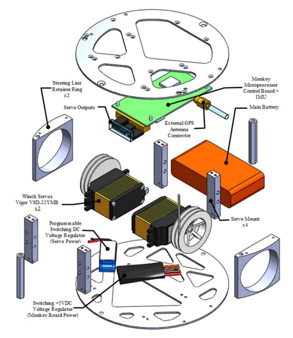
Figure 16. New, miniaturized System V.2 steering control system architecture (exploded view).
