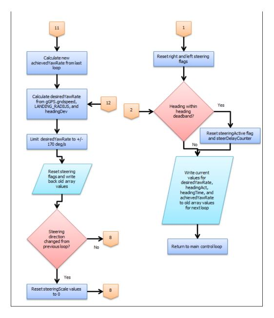
Figure 29. (Previous page and this page.) Flow chart of the landing routine of the System V.2 control software.
