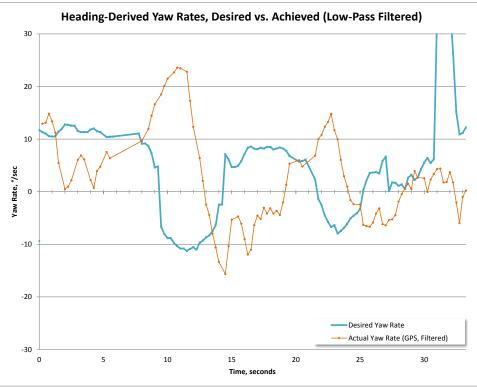
Figure 45. (5 plots, above) Flight performance data for the second iteration of the steering software, in calm wind conditions. As can be seen in the first plot, the parafoil system landed within a meter of its target coordinates. Unfortunately, this behavior was not repeatable in the presence of even a moderate breeze.
