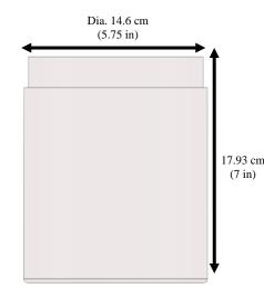
Figure 13. Dimensions of parafoil return system volumetric envelope, as required by the Payload Containment and Thermal Control Unit (PCTCU).
