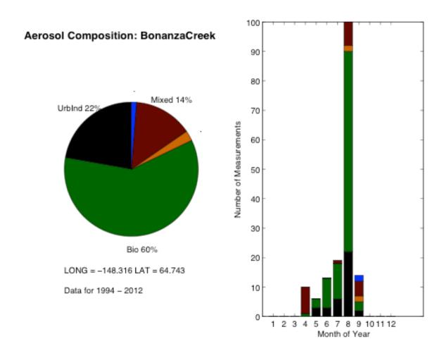
Bonanza Creek is a rural region about 30 km downwind from Fairbanks Alaska. The aerosol is mainly biomass burning. The prevailing winds in August are towards or away from Fairbanks, perhaps due to the fact that the instrument at Bonanza Creek is in a valley oriented towards Fairbanks. In August 2004 and 2005 the smoke from numerous forest fires covered the sky above Bonanza Creek.
