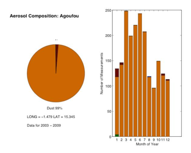
The sun photometer site is located on a sand dune near the village of Agoufou in Mali. Our Mahalanobis calculations used more than a thousand inversions over a seven-year period and indicated that the aerosol is nearly all dust.
