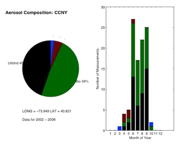
CCNY stands for City College of New York. The instrument is located on top of a building in New York City. This is in a heavily urbanized area. The identification of biomass burning aerosol is difficult to explain. Scatterplots of SSA vs EAE indicate the presence of a significant number of observations in which the Single Scattering Albedo is less than 0.85. Our urban industrial reference cluster assumes SSA greater than 0.9. These "outliers" are identified as biomass. See scatterplot below.
