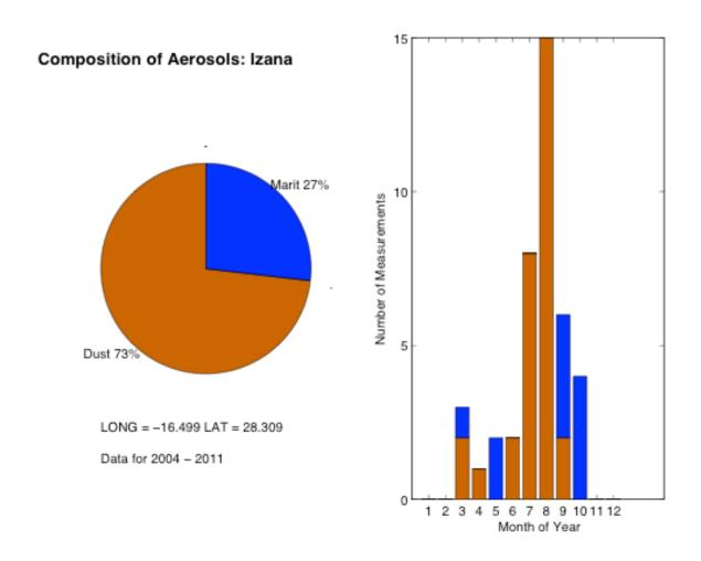
Izana is an observatory on top of a mountain (at 2367 meters above sea level) on the island of Tenerife (Canary Islands). This location is free from local anthropogenic aerosols and is used for calibration of the Cimel sun photometers. The summer months are dominated by dust aerosol, whereas maritime aerosol prevails during the fall. This site is in the transport path of the Saharan Air Layer, which can transport dust from African sources westward.
