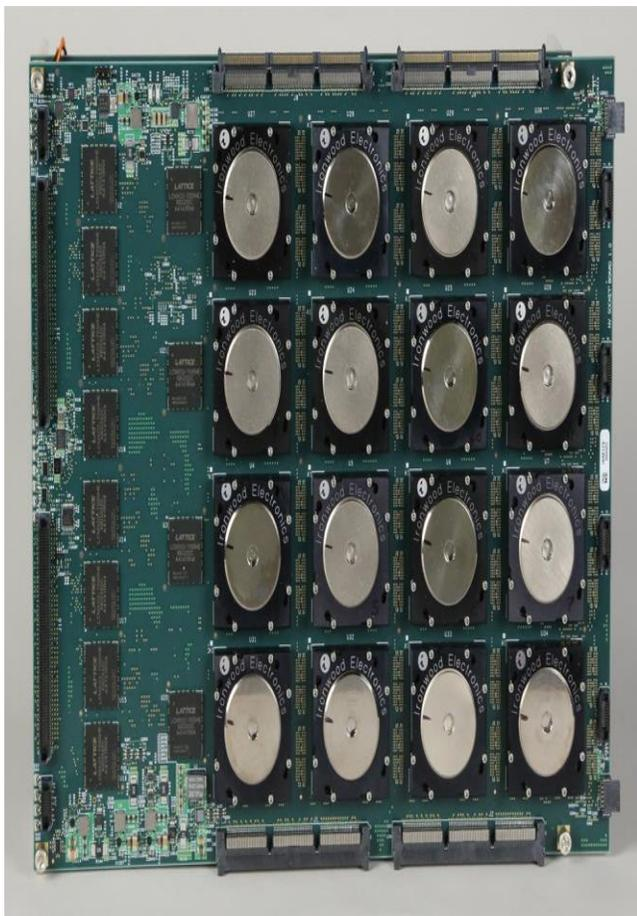
**Figure 1:** IBM's 4x4 array of SyNAPSE chips each one with 1 million electronic neurons and 256 million electrical synapses between them<sup>[7]</sup>
