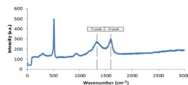
Figure 3. Raman spectra of Si/C active material. A greater G-peak relative to D-peak suggests a graphitic carbon layer.
