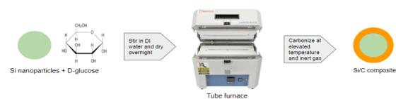
Figure 1. Synthesis of Si/C active material .
