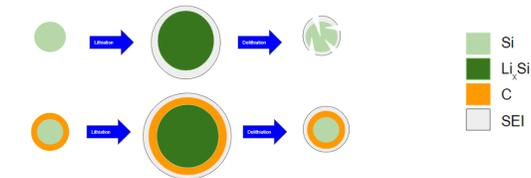
Figure 2. Electrode behavior during cycle of Si only (top), and Si/C (bottom). The Si only electrode is prone to self-pulverization after severe expansion during lithiation.
