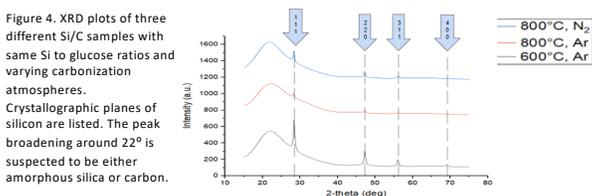
Figure 4. XRD plots of three different Si/C samples with same Si to glucose ratios and varying carbonization atmospheres. Crystallographic planes of silicon are listed. The peak broadening around 22° is suspected to be either amorphous silica or carbon.
