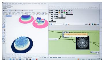
At the March 2023 3D printing workshop at Chopsticks Alley Art, a participant's computer screen displays the original 2D image alongside its 3D counterpart in Grasshopper software, a significant step of the design process. The finalized 3D design is then saved and converted into a 3D-printed sculpture.
