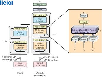
An example of vector operation optimization integration within a deep neural network transformer architecture. The left side represents an example of a neural network transformer architecture, and the right side shows the Dr. Guzun Laboratory's contribution, where they optimize vector operations such as dot-products through novel quantization and compression approaches. Image courtesy of Dr.
