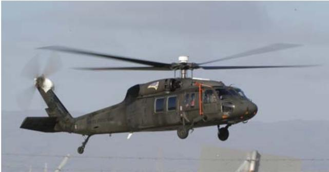
**Figure 3. The RASCAL JUH-60A In-Flight Simulator**
