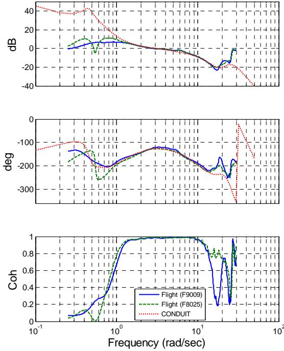
**Figure 4 – Lateral broken loop response comparison between analysis and flight**
