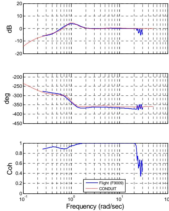
**Figure 7 – ACVH longitudinal ground speed disturbance rejection response comparison between analysis and flight**
