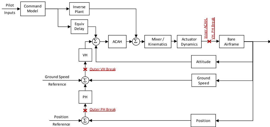
**Figure 13 – Inner and outer loop break locations for stability margin calculations**
