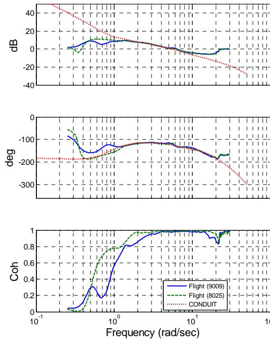
**Figure 5 – Directional broken loop response comparison between analysis and flight**
