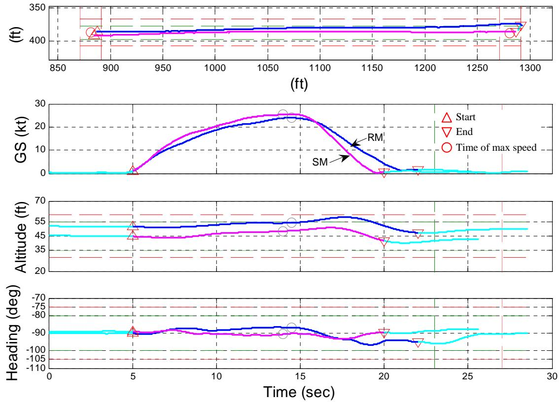
**Figure 22 – Sample Lateral Reposition results for both cases**
