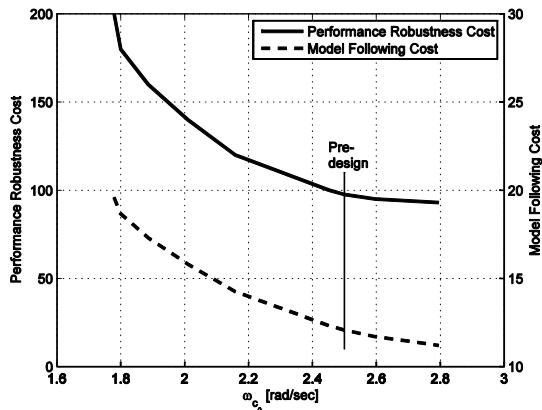
Figure 8 – Variations in model following and performance robustness with changes in crossover frequency (from reference [12])
