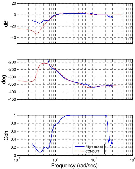
**Figure 6 – ACAH lateral disturbance rejection response comparison between analysis and flight**
