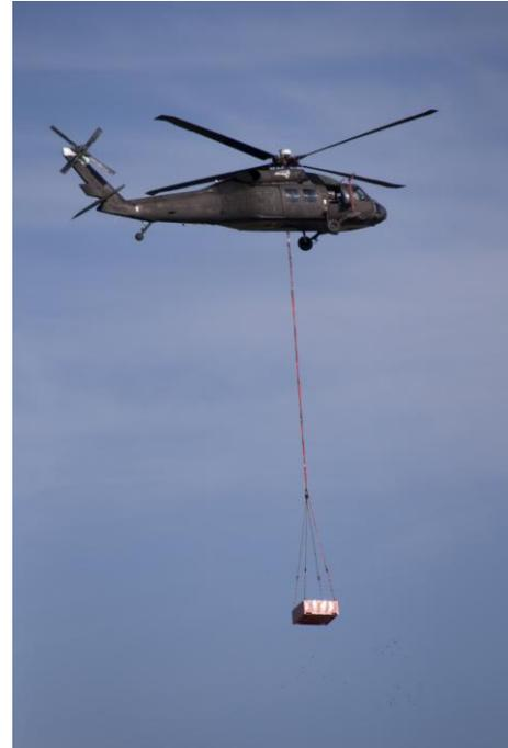
**Figure 1. JUH-60A RASCAL helicopter with external load.**
