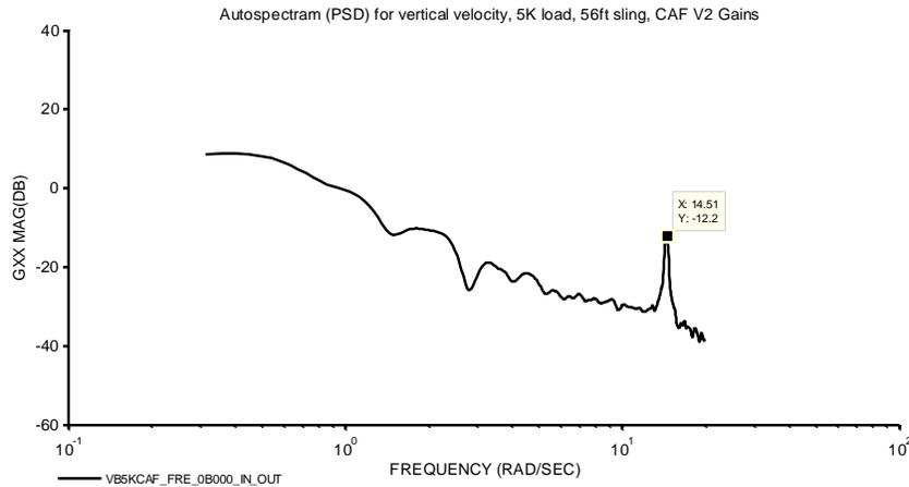
**Figure 19. Autospectrum for vertical velocity from flight.**
