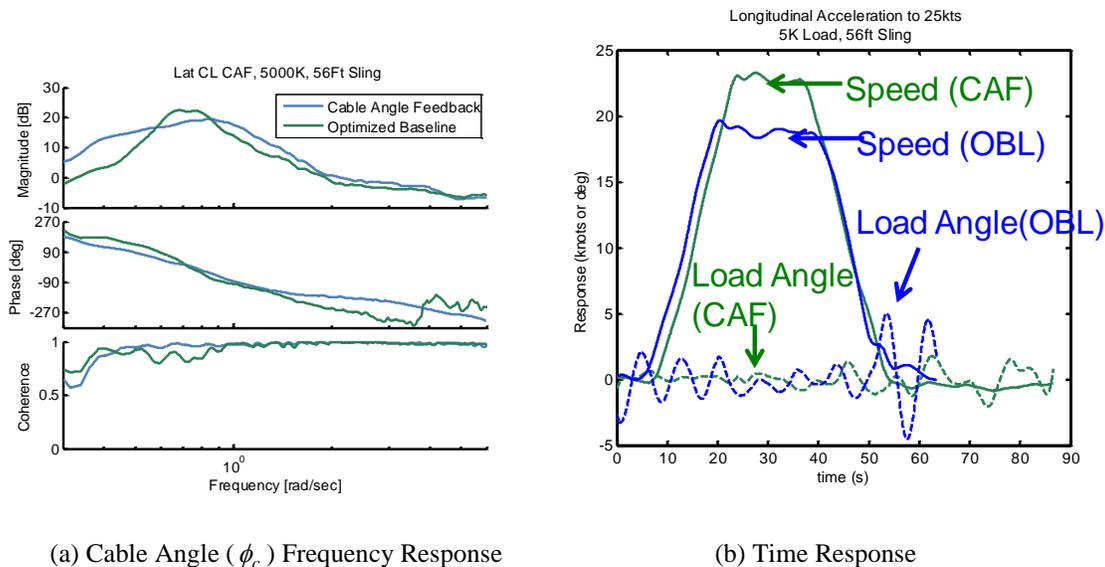
Figure 23. Flight load response, PH mode (5K, 56ft sling).
