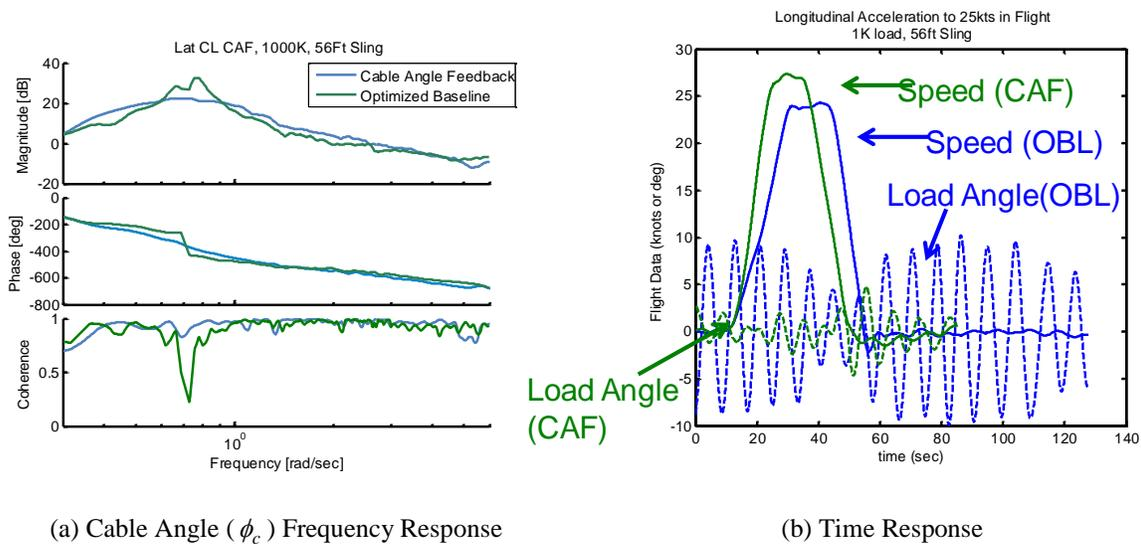
Figure 24. Flight load response, PH Mode (1K, 56ft sling).
