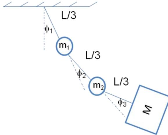
Figure 16. Sling model with 3 segments.
