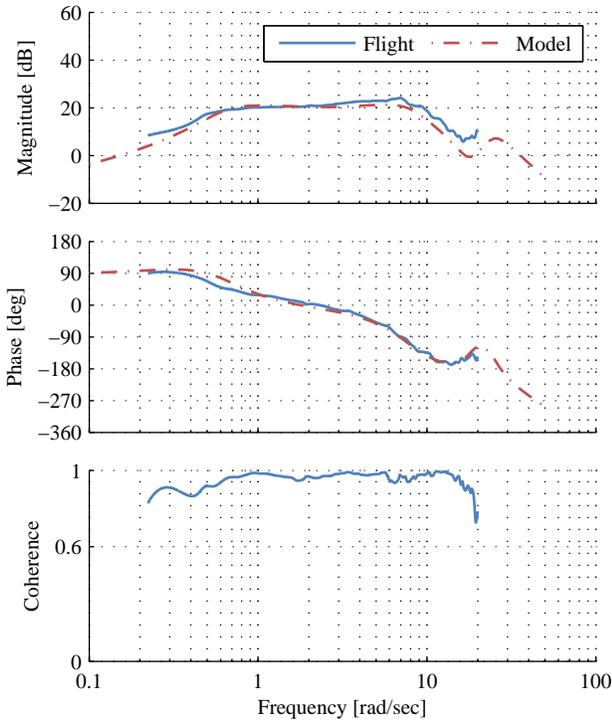
**Fig. 3: Roll axis closed-loop validation**  $\left(\frac{p}{\delta_{lat}}\right)$
