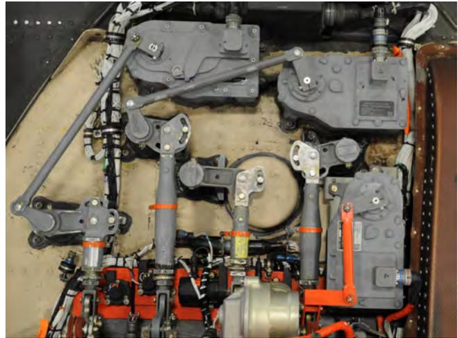
**Fig. 6: AFDD's EH-60L trim actuators (clockwise from top left: yaw, roll, collective)**
