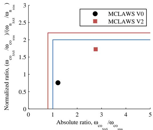
**Fig. 4: Yaw axis actuator command cutoff frequency allocation specification**
