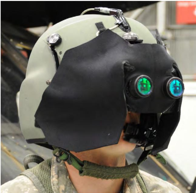
**Fig. 13: Modified night vision goggles and shroud to simulate DVE conditions**
