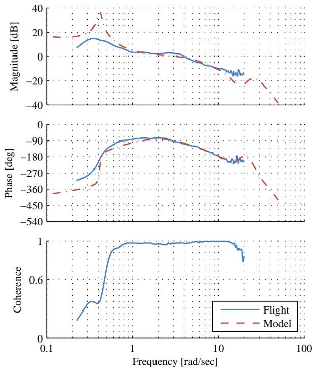
Fig. 2: Roll axis broken-loop validation
