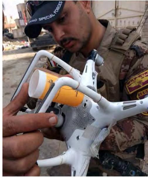
**Figure 2. Weaponized commercial quadrotor.**
