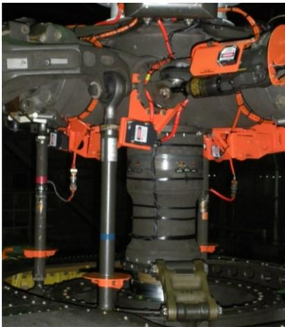
Figure 2. Rotor blade measurement system [12].
