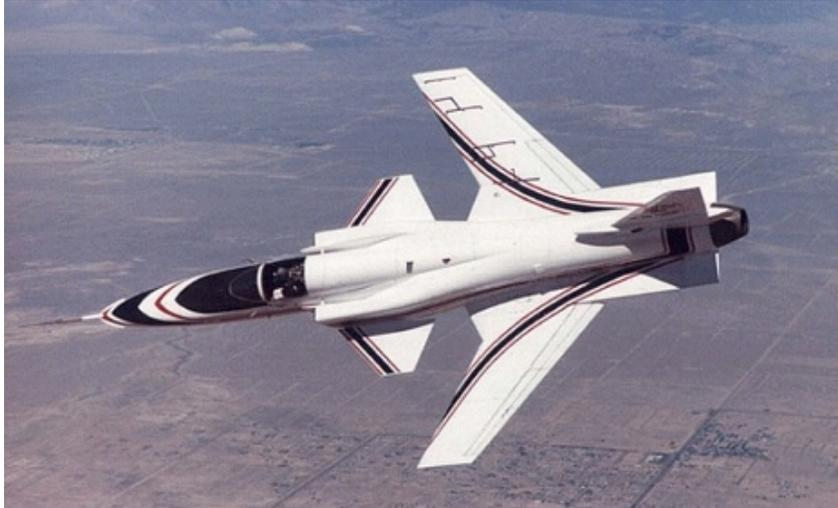
Fig. 17 X-29A forward-swept wing fly-by-wire demonstrator.
