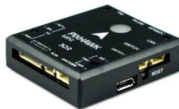
**Figure 2. Pixhawk Mini Autopilot Controller Board.**
