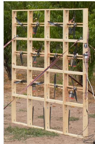
Fig. 19: Gust wall with 12 fan cells.
