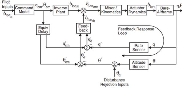
Figure 4: 2DOF Controller Architecture, reproduced from Ref. 12
