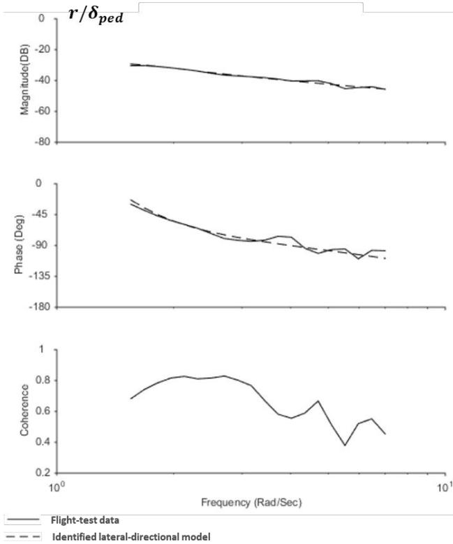
**Figure 8. Lateral-directional frequency response – yaw rate to pedals**
