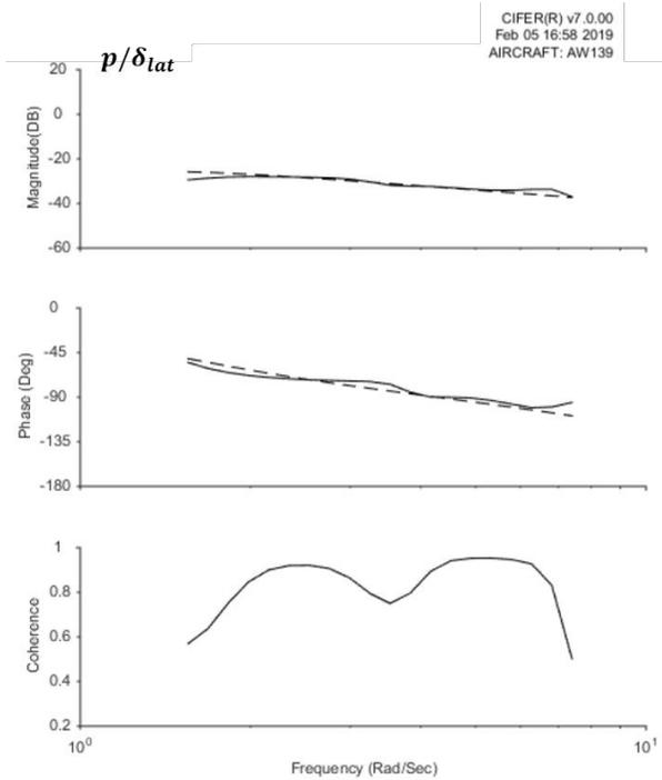
**Figure 5. Lateral-directional frequency response – roll rate to lateral stick**
