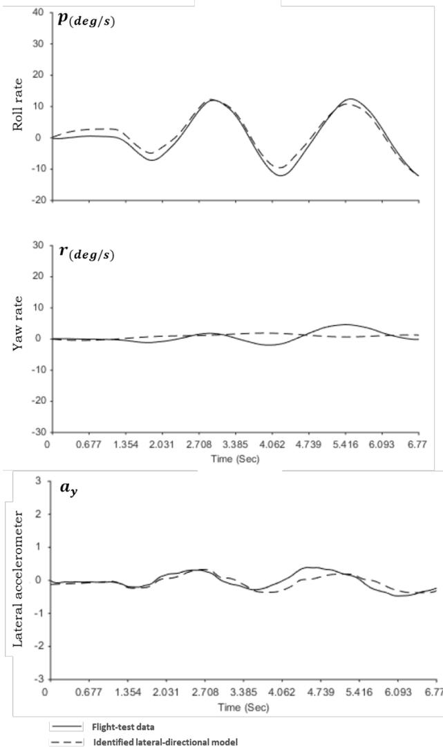
**Figure 9. Lateral-directional model time-domain verification agreement for a lateral stick input**
