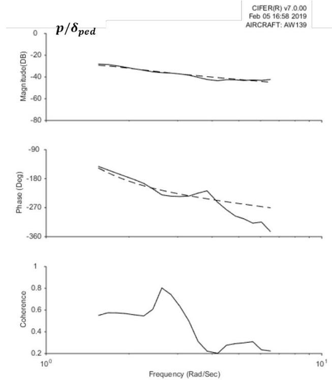
**Figure 7. Lateral-directional frequency response – roll rate to pedals**
