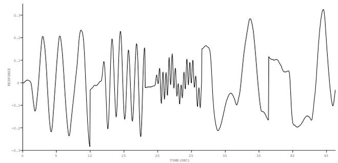
Figure 4. Roll rate response ( $p, \text{rad/sec}$ ) for 5 QTG flight-test records.
