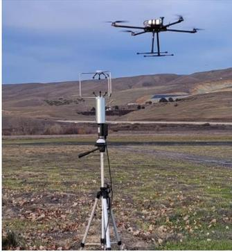
Figure 3. Flight Testing Set-up
