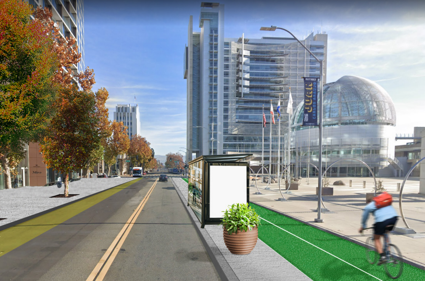
Figure 25. Before and After Rendering of E. Santa Clara Street Optimized for AV with Bike Lane and Pick-Up and Drop-Off Zone. Source: Author
