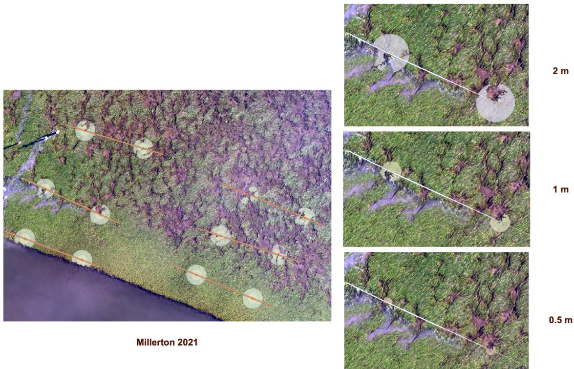
Figure 13. Left: The result of the buffer zone generations on the sampled points and the outcome of the “Intersect” and “Dissolve tools” alongside the digitized transect lines and sampled points. Right: Close-up view of the intersection between the buffer polygons and the eelgrass areas at 2, 1, and 0.5-meter radius.
