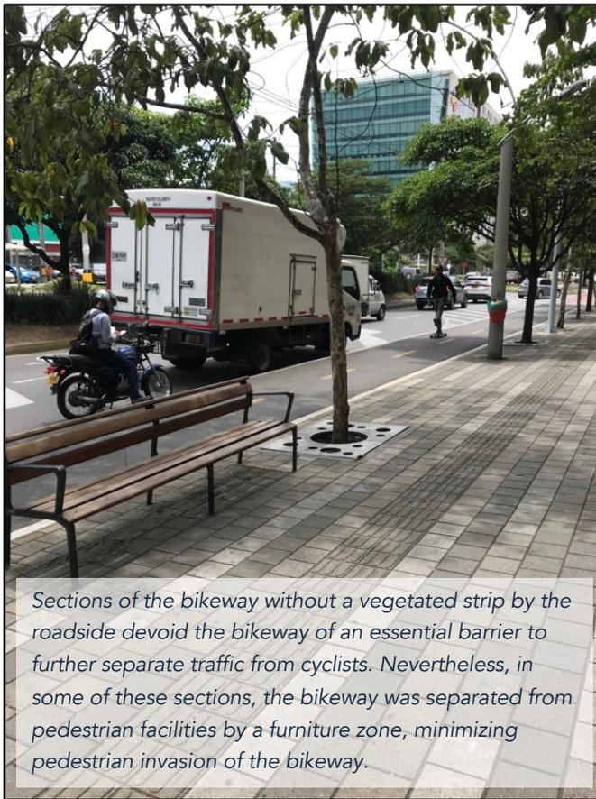
*Sections of the bikeway without a vegetated strip by the roadside devoid the bikeway of an essential barrier to further separate traffic from cyclists. Nevertheless, in some of these sections, the bikeway was separated from pedestrian facilities by a furniture zone, minimizing pedestrian invasion of the bikeway.*
