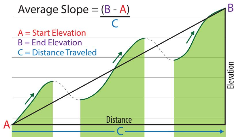
Figure 4.2. Representation of average slope.
